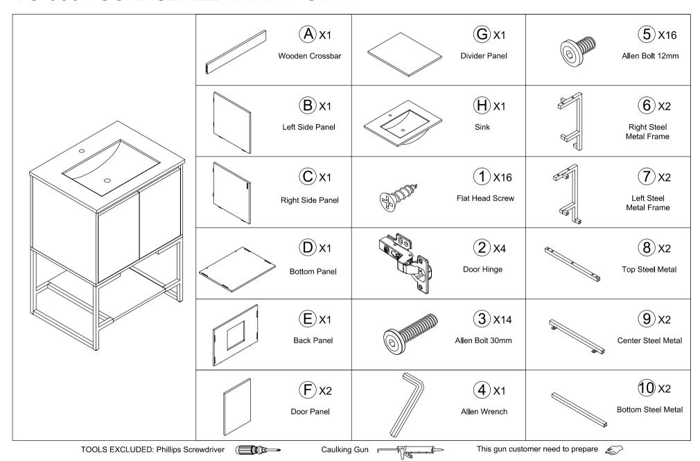
Step 1. Attach the steel metal bars (8,9,10) to the right steel metal frame (6) and the left steel metal frame (7) by using the Allen bolts 30mm (3) and the Allen wrench (4).
