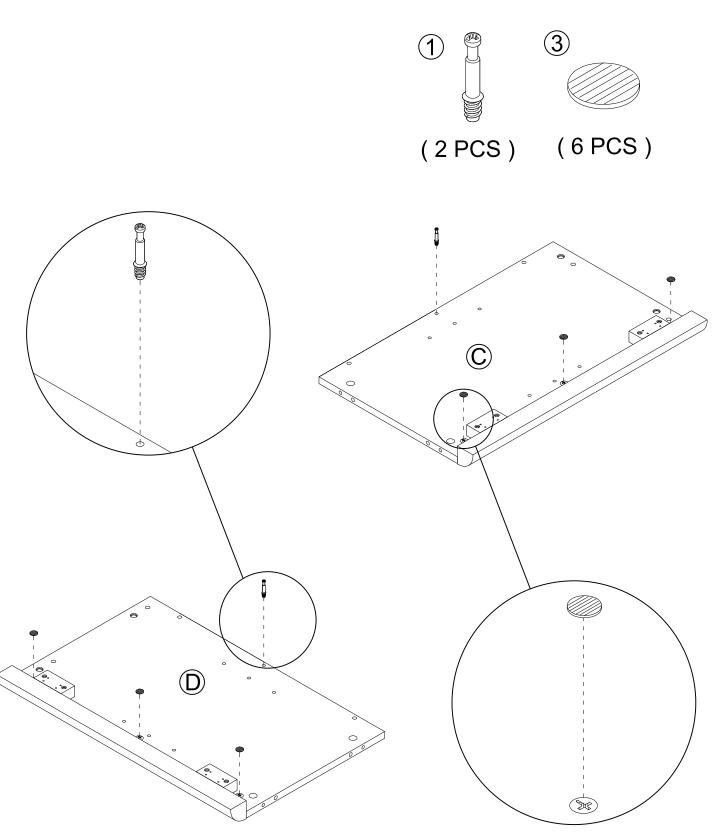
\* Attach the LEFT PANEL (C) and RIGHT PANEL (D) to the ASSEMBLY by the Two KD CAM (2), Two COVER CAP (3), Four WOOD DOWEL (4) and
