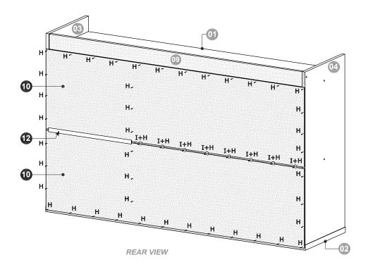
• Connect Back Panels (10) with nails (H), metallic plates (I) and plastic profile (12).
