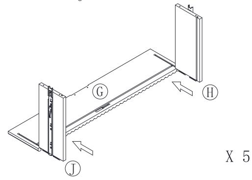
♦ Slot the DRAWER BOTTOM SUPPORT (O) to the DRAWER FRONT (G).
