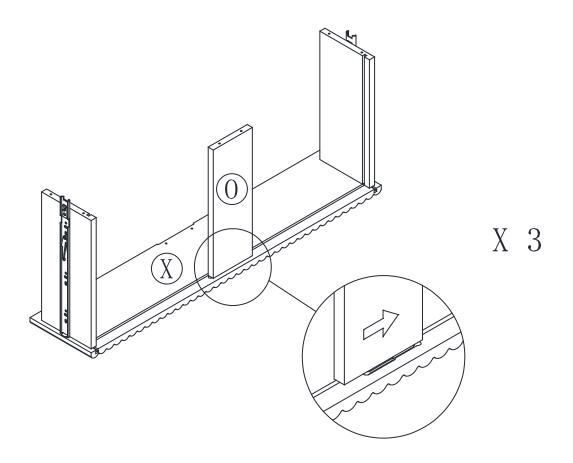
Slide the DRAWER BOTTOM (M) into the grooves, in the DRWAER SIDES (S and R), and the DRAWER FRONT (X).
