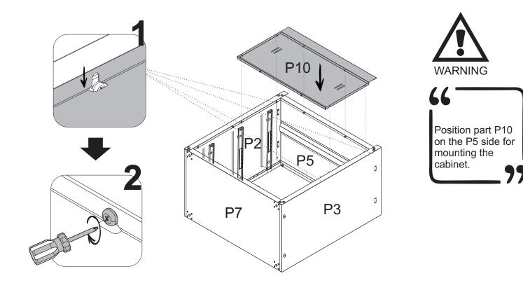
2 - Fit parts **P2** and **P3** to parts **P5** and **P7** with **F1** and **F2**.
