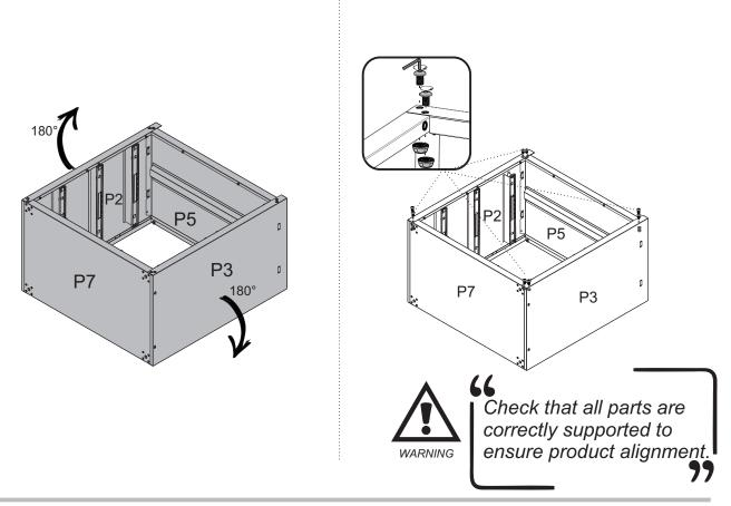
**STEP 4** 1 - Fit part **P10** into parts **P2**, **P3** and **P5**. Check that all fits are supported over the bolts. 2 - After fitting the parts, screw the bolts until locked.
