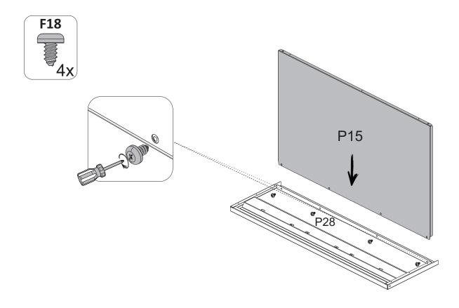
**STEP 8** 1 - Align parts **P12** and **P13** to part **P15**, until it leans against piece **P28**. 2 - Screw the two with **F1**8.
