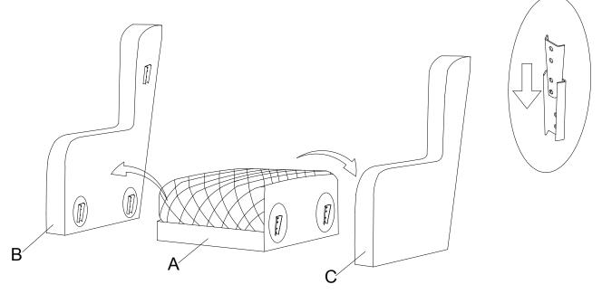
Step 2: Attach Backrest(D) to Left arm(B) and Right arm(C)
