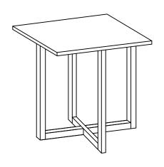
Caution:Please do not tighten all bolts until the end table is completely assembled!
