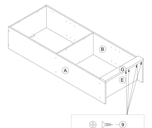
1/2" FLAT HEAD SCREW (8 used in this step)
