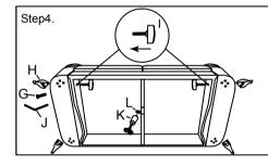
Screw down Bolt(I) as shown, Then Attach Legs(H) and Middle Leg (K) to the bottom with Bolt (G) and Allen key (J) as picture shows.
