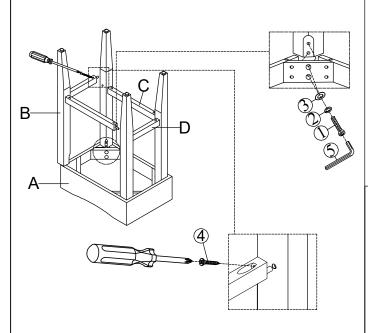
Ensure screw holes in stretchers face as shown on diagram. If stretchers are properly oriented, once stool is turned upright, screw holes will face toward floor.
