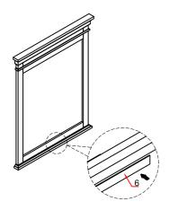
Follow the customer's request and attach felt fabric to the underside of mirror (bottom touching the top of dresser).
