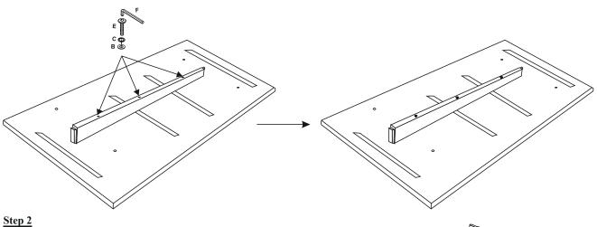
Attach two Metal Corner Brackets G to the inside and outside of each panel of the Leg Assembly using a Short Bolt D, Lock Washer C, and Large Flat washer A. Do not fully tighten at this point.
