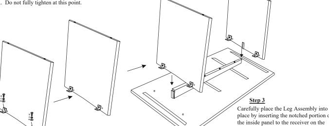
place by inserting the notched portion of the inside panel to the receiver on the Support Stretcher. Keep Leg Assembly
