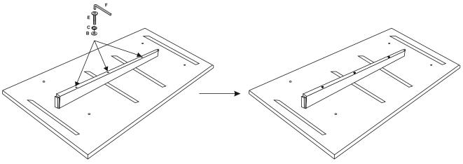
Attach two Metal Corner Brackets G to the inside and outside of each panel of the Leg Assembly using a Short Bolt D, Lock Washer C, and Large Flat washer A. Do not fully tighten at this point.
