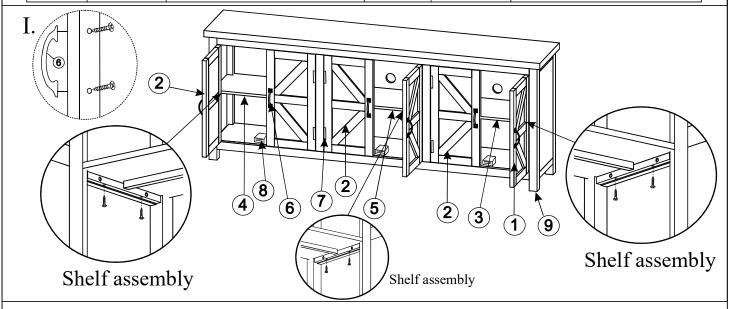
PLEASE NOTE: To help prevent the possibility of tip-over, install the tipover restraint provided.
