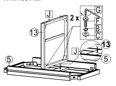
Carefully lay the Shelf Unit on the side and attach a Right Side Leg and a Left Side Leg to the top corners using a Bolt (E), a Lock Washer (B) and a flat Washer (C).
