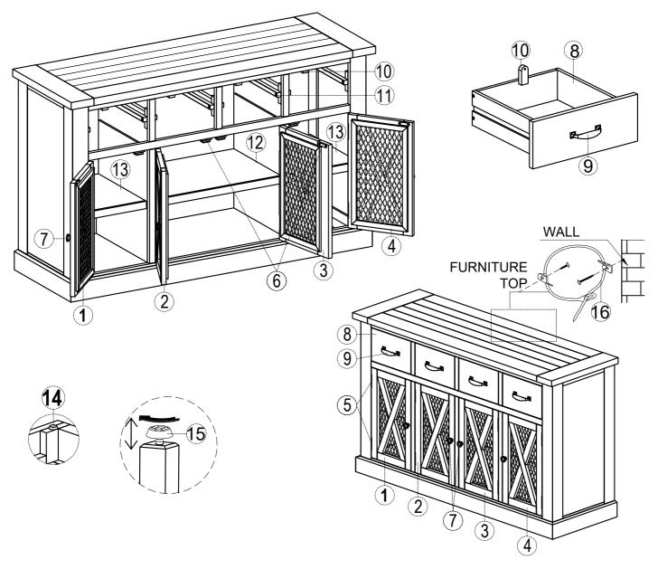
PLEASE NOTE: To help prevent the possibility of tip-over. Install the ANTI- TIP OVER restraint provided.
