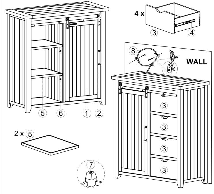
PLEASE NOTE: To help prevent the possibility of tip-over, install the ANTI- TIP OVER restraint provided.
