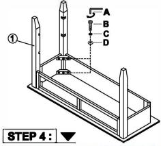
Carefully turn the assembled table to the upright position. Put back the drawer. Attach the Anti-tip Over restraint. Assembly is now complete.
