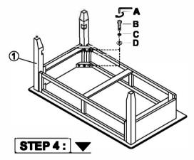
Carefully turn the assembled table table to the upright position. Put back the drawers. Assembly is now complete.
