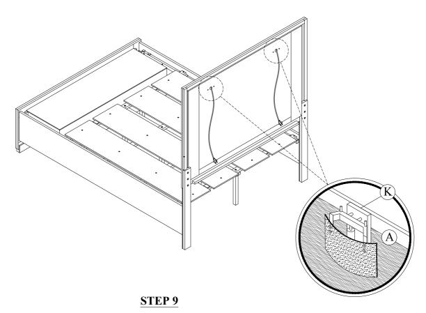
Install the Lamp Set according to the assembly instruction inside the Lamp Box. Then, align and attach the Lamp at the top of Headboard (A).
