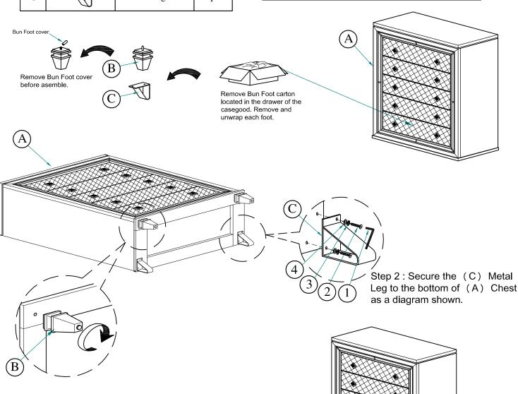
Step 1 : Secure the (B) Bun Foot to the bottom of (A) Chest as a diagram shown.
