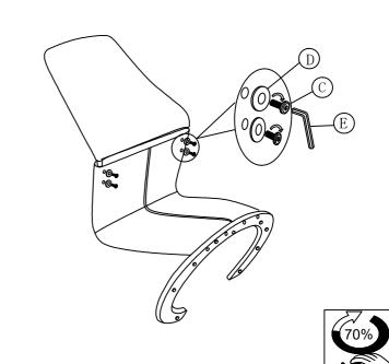
Step 2-b:Press the backrest(B) harder to make inner surface of the back close contact with the seat(A) and then 100% lock the four bolts(C). (Note: do not lock the screws when the back and cushion are at untight contact position like poor assembly picutre)
