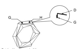
Step1: Put the Aluminum cake(H) on the Stainless steel pillar(B) by screw(G)
