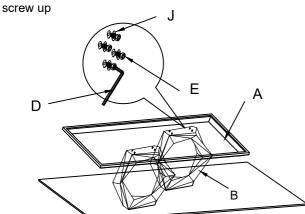
Step 3:Turn over,use screw (E) connect the stainless steel base (B) with the stainless steel base (A) by Allen key (D).
