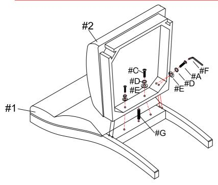
DO NOT FULLY TIGHTEN ALL BOLTS (#A,C) UNTIL THE FULL ASSEMBLY IS COMPLETED
