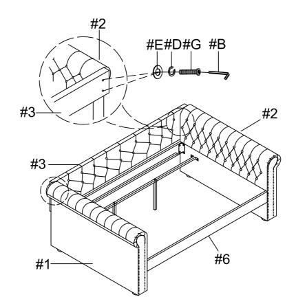
Prepare 4 bolts assembly by inserting lock washer (#D), then flat washer (#E) onto bolts (#G). Align back rest (#3) to the holes of the arms (#1,2). Secure with bolts (#G).
