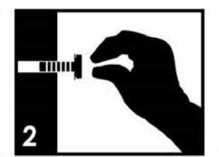
Position each part correctly and insert screws or bolts into their respective holes by hand tighten or using the proper hand tool. Only tighten when step is completed or when instructed to do so.
