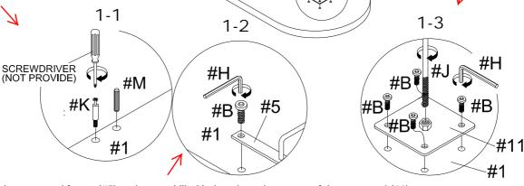
2. Align the top panel frame (#5) to the pre-drilled holes along the center of the top panel (#1). Insert a total of 6 bolts (#B) along the sides and secure using the Allen wrench (#H).
