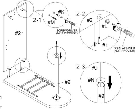
Insert two cam locks (#L) into the large pre-drilled holes along the side of the side panel (#2).
