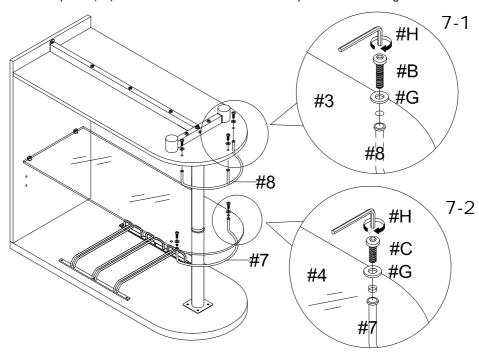
2. Prepare 2 bolt assemblies by inserting a flat washer (#G) onto bolts (#C). Then align the glass shelf guardrail (#7) to the pre-drilled holes on the bottom of the glass shelf (#4). Insert bolt assemblies from the top and secure using the Allen wrench (#H).
