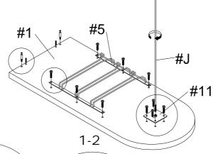
Align the bracket (#11) to the four pre-drilled holes near the curved end of the top panel (#1). Insert stud bolt (#J) into center hole, turn right to tighten. Insert 4 bolts (#B) to the corner holes and secure using the Allen wrench (#H).
