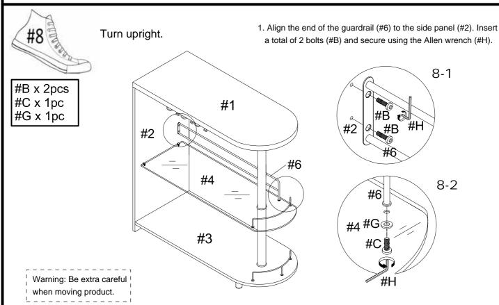
2. Align the other end to the pre-drilled hole on the glass shelf (#4) Insert a flat washer (#G) onto bolt (#C), then insert bolt assembly into hole and secure using the Allen wrench (#H).
