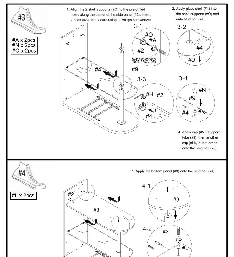
2. Insert two cam locks (#L) into the large pre-drilled holes along
