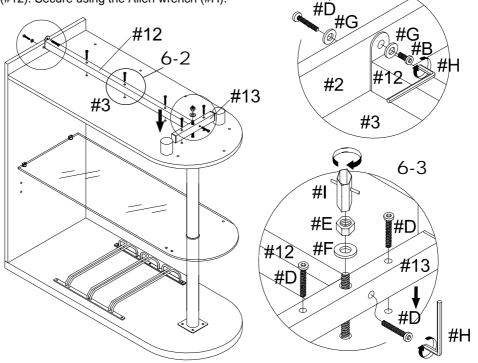
3. Apply bottom support tube B (#13) onto the stud bolt (#J). Apply a flat washer (#F) then hex nut (#E) onto the stud bolt (#J), in that order. Secure using the wrench (#I). Insert a total of 3 bolts (#D) into the remaining holes on (#13) and secure using the Allen wrench (#H).
