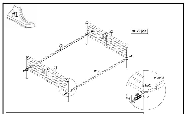
Align the upper rear and front tubes (#9,10) to the holes along the upper headboards (#1,2), then insert the bolts (#F) into each hole. Secure using the Allen wrench (#H).
