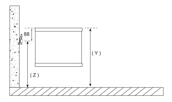
Please use minimum 2 holes on Medium Bracket and Long Bracket, and minimum 1 hole, to apply the wall plug and screw. Use additional holes when necessary.
