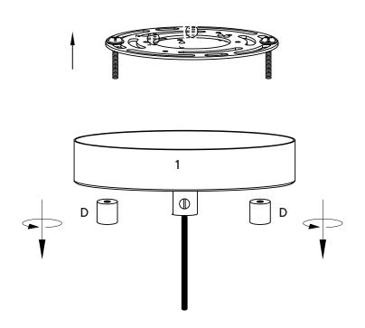
Determine your desired total drop of the Lamp Cord (2). The total drop is the distance from the ceiling to where you would like the bottom of the pendant to hang. Once decided, secure the Lock Sleeve (F) at the Ceiling Canopy (1).
