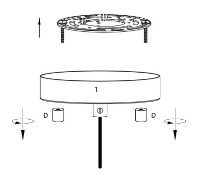
Determine your desired total drop of the Lamp Cord (2). Total drop is the distance from the ceiling to where you would like the bottom of the pendant to hang. Once decided, secure the Lock Sleeve (F) at the Ceiling Canopy (1).
