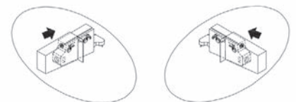
11.9 Once the cabinet is installed and adjusted, install the latch covers.
