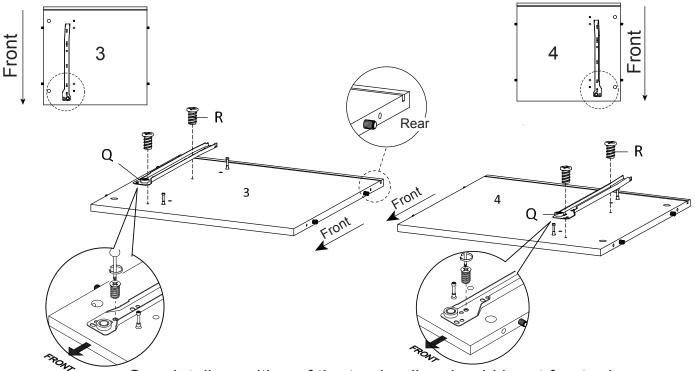
See details position of the track roller should be at front edge
