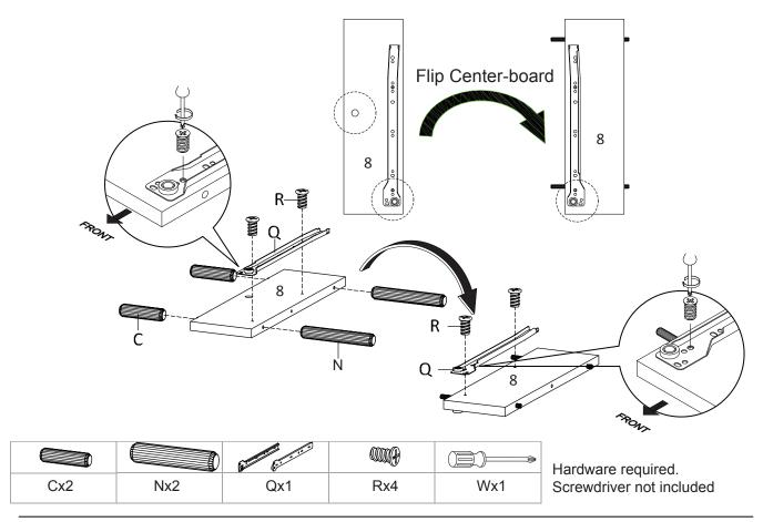
STEP 8: Securing the Center Board (8) to Fixed Shelf (12)
