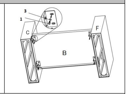
Attach the Seat Part(B) by using 8 pcs of M6\*20 Screws(1) and 8 pcs of M6 Flat Washer(2) as picture. Tighten all screws with Allen Key(4).
