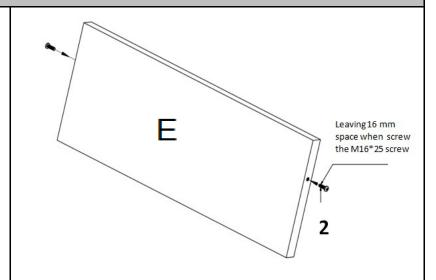
Screw the M6\*25 Screw onto the Back Part(E). Be sure not over-tighten. Need to leave 16mm exposed length on the M6\*25 Screw after screwing.
