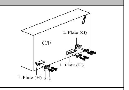
Attach the L Plate (Hand G) onto each Armrest (C and F) by using 6pcs of M6\*20 Screw(1) and M6 Flat Washer(3). Tighten all screws with Allen Key(4). Repeat on the other Armrest(F)
