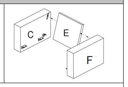
Joining the Back Part(E) with the Armrest(C and F) by inserting the exposed M6 Screw on the Back Part into the hole on each Armrest.
