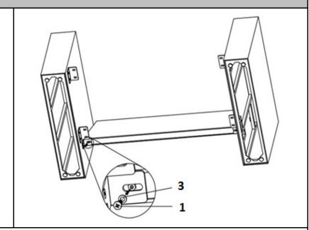
Put the M6\*20 Screw(1) and M6 Flat Washer(3) on the L Plate(H and G) on the Armrest. Tighten all screws with Allen Key(4).
