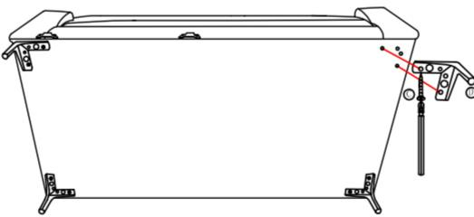
Note: Take out the legs and screws from the small box and screw the legs at the proper position of the bottom
