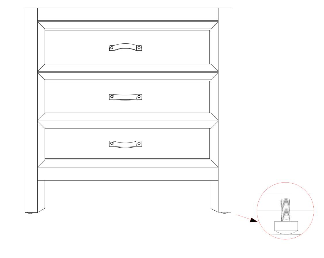
Note: Levellers are provided at bottom to balance the product on uneven surface.
