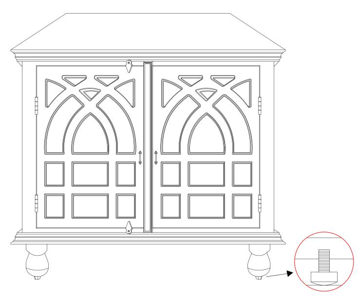
Note: Levellers are provided at bottom to balance the product on uneven surface.
