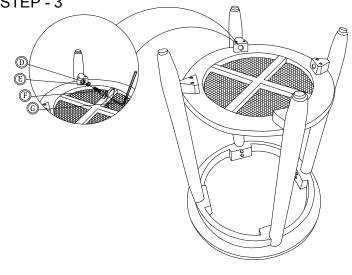
Install the shelf (C) on the legs according to the hole in the leg, Install the JCBC M6 x 40 (F) along with the washer (D) and spring washer (E), (tighten with an allen key (G))
