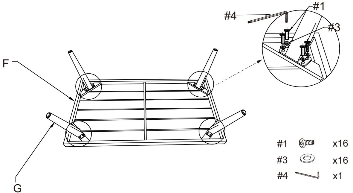
Step 5. Carefully turn assembled unit upright on a flat surface.
