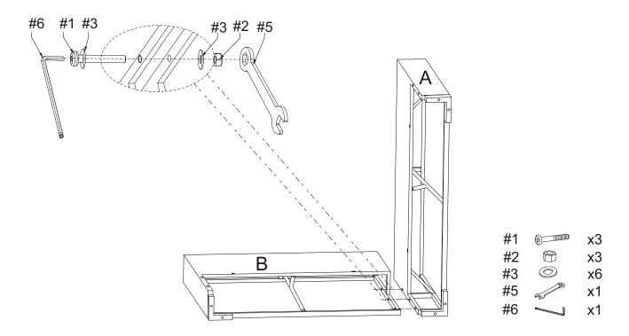
Step 2. Attach seat panel (part C) to assembled unit (parts A&B) using bolts (part #1), washers (part #3), nuts (part #2), wrench (part #5) and allen key (part #6).
