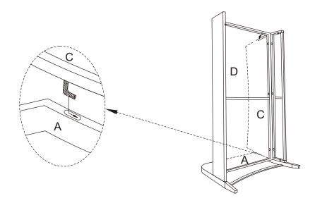
Step 3. Attach back panel (part C) to assembled unit (parts A & D) using short bolts (part G), flat washers (part J) and allen wrench (part L).
