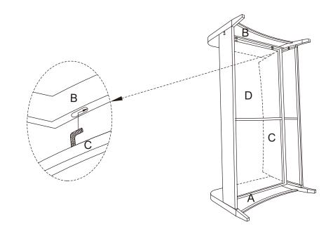
Step 5. Attach right arm panel (part B) to assembled unit (parts C & D) using short bolts (part G), long bolts (part H), flat washers (part J), hex nuts (part I), wrench (part K) and allen wrench (part L). NOTE: Please fully tighten all bolts at this time.
