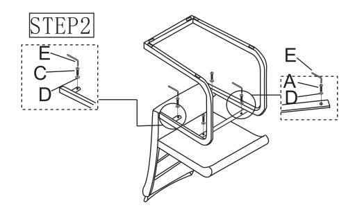
Note:Please do not tighten all bolts until the item is fully assembled.Once assembled tighten all bolts.
