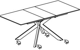
ADJUST THE GLIDES UNDERNEATH TO BALANCE THE TABLE
