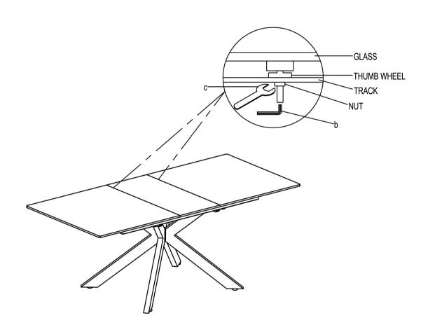
A. IF THE EXTENSION LEAF IS NOT LEVELED TO THE SIDE TOPS, PLEASE USE WRENCH c TO LOOSE THE 4 NUTS UNDERNEATH THE EXTENSION LEAF, AND TURN THE THUMB WHEELS TO LEVEL THE LEAF TO SIDE TOPS. FASTEN THE NUTS AFTER ADJUSTED.
