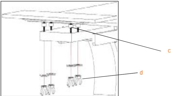
Note : before fully tighten "d", please move the extension marble more left or right , or adjust "c" to make it more up or down so that the extension can be align with the middle marble well.
