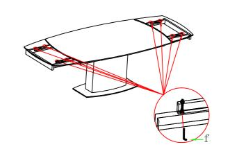
Turning the thumb wheel to adjust the length of the bolt to make the side glass on the same level line with the middle glass.
