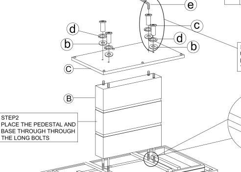
STEP3 USE THE ALLEN KEY TO FASTEN THE NUTS AND WASHERS TO THE BOLTS
