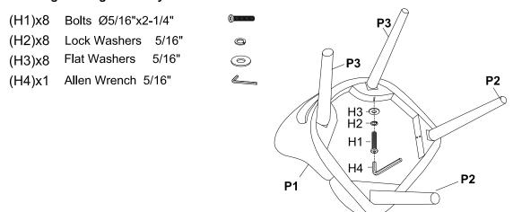
ADDITIONAL NOTE ABOUT SAFETY: BOLTS MAY LOOSEN DURING NORMAL EVERYDAY USE. THEY SHOULD BE PERIODICALLY INSPECTED AND RE-TIGHTENED TO PREVENT DAMAGE OR INJURY. ALWAYS CHECK TO ENSURE THAT ALL HARDWARE IS KEPT TIGHTENED.
