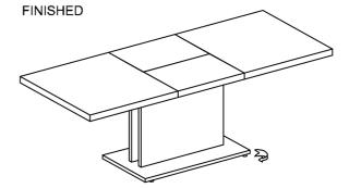
Adjust the glides underneath to balance the table.
