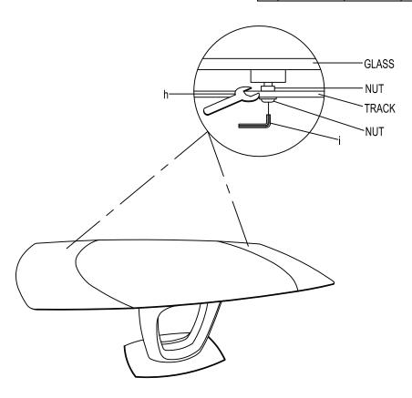
A. IF THE EXTENSION PANNEL IS NOT LEVELED TO THE TABLE TOPS, PLEASE USE h TO LOOSE THE 4 NUTS UNDERNEATH THE TRACK, AND USE I TO TURN THE NUTS TO LEVEL THE SIDE PANNEL WITH TABLE TOP. FASTEN THE NUTS AFTER ADJUSTED.
