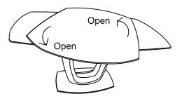
Extend by anti-clockwise rotating, and close byclockwise rotationg
