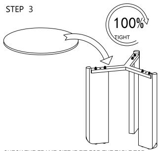
CHECK THE FRAME SIZE IF FIT FOR THE TABLE TOP THEN REMOVE THE TABLE TOP AND 100% TIGHT THE ALL THE SCREWS ON THE FRAME.
